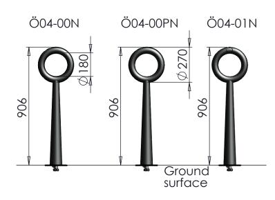
Hoop with soleplate for mounting above ground. The soleplate is used in the case that the foundation cannot be dug.
